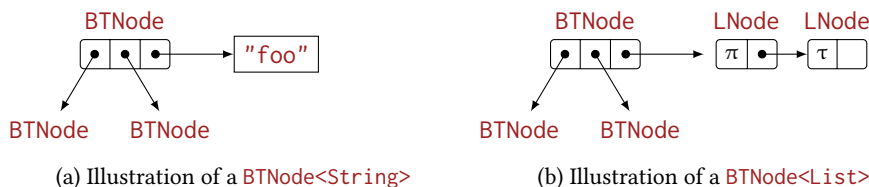
Figure 5.1: Generics influence the number of potential roots a type has, as shown here with a binary tree node BTreeNode<T> . The String does not contain a root, but a node in a linked list LNode does.
